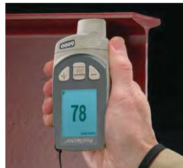
Flip Display enables right-side-up viewing
