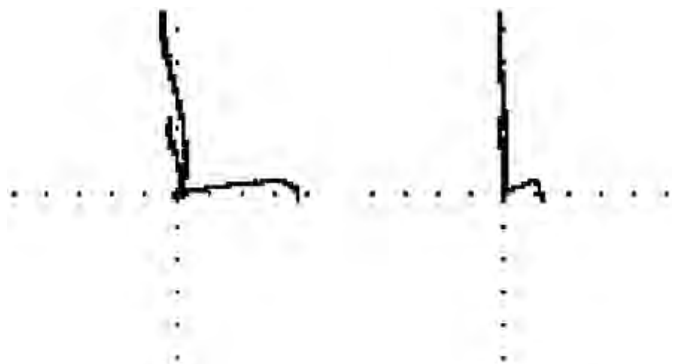
Probe traversed along toe of weld with defect (positive signal)
