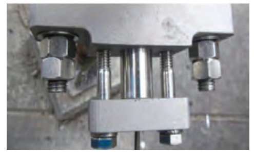
7MHz Ultra High-Temp Delay Line: transducer and mounting clamp for continuous 500°C (932°F).
