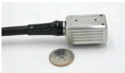
10MHz PAUT Dual: special 64-element dual for HTHA exams.
