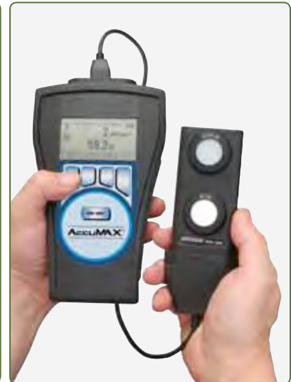
XR-1000 readout unit with dual-wavelength sensor detector connected to unit via USB cable
