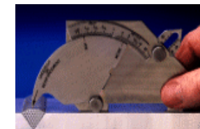
BRIDGE CAM GAGE Measures angle of prep, Excess weld metal, Undercut depth, Pitting depth, Fillet weld throat size, Fillet weld length, Outside alignment DETEK P/N VWG-003
