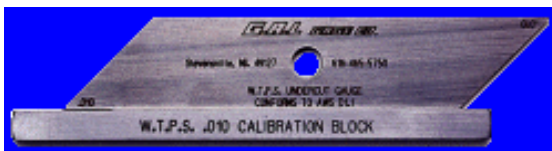
W.T.P.S. TYPE GAGE Measures .010" deep undercut to tolerances +/- .0005" DETEK P/N VWG-004
