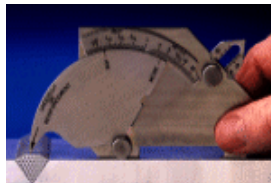
BRIDGE CAM GAGE Measures angle of prep, Excess weld metal, Undercut depth, Pitting depth, Fillet weld throat size, Fillet weld length, Outside alignment DETEK P/N VWG-003
