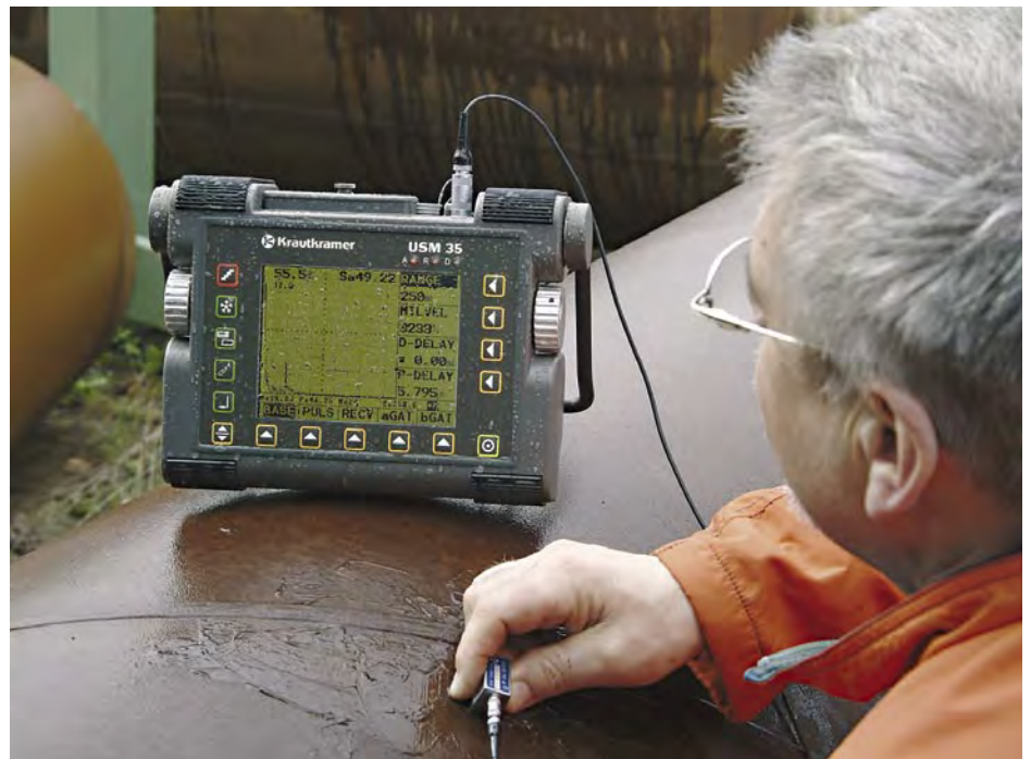
Inspection of a weld
