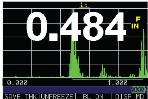
ECHO 9W – Includes Waveform, Coating Thickness
